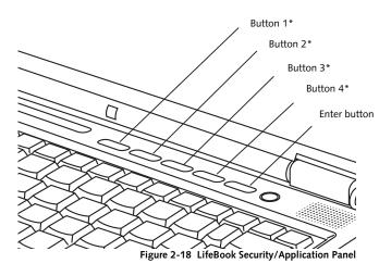
\* Security/Application Launcher buttons (for entering passwords and launching applications)
